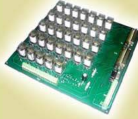
Custom Built Relay Module
